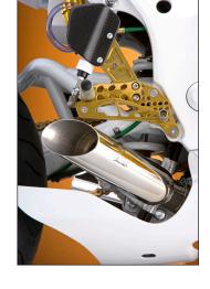
■Holey rearsets, 'Busaman! Gold-anodized foot controls by Gilles Tooling are drilled and machined wherever possible to reduce weight. Simple little Voodoo mufflers slip onto snowwhite ceramic-coated headers.
