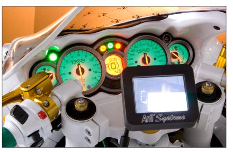
■Green lighting theme continues with instruments treated to a graphic re-do by CSC. AnT Systems Rear-View monitor means no ugly mirrors. Generous use of white paint and powdercoat brightens the entire cockpit area. (Below) Green kanji lettering lights up any time the ignition is on.
